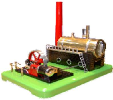
**Steam engine** is polytechnic toy, which presents mock-up real steam engine and working same principle. It is possible it use for drive model machine. Turning machinery is in both directions. On base is fixation hearth with steam-boiler, furniture fittings and support with steam cylinder and divorce and crank mechanism. Vapor goes through pipe to kettle-drums. We use dried spirit (esbit) as fuel (or warming gel for camping "Ecoflame").
